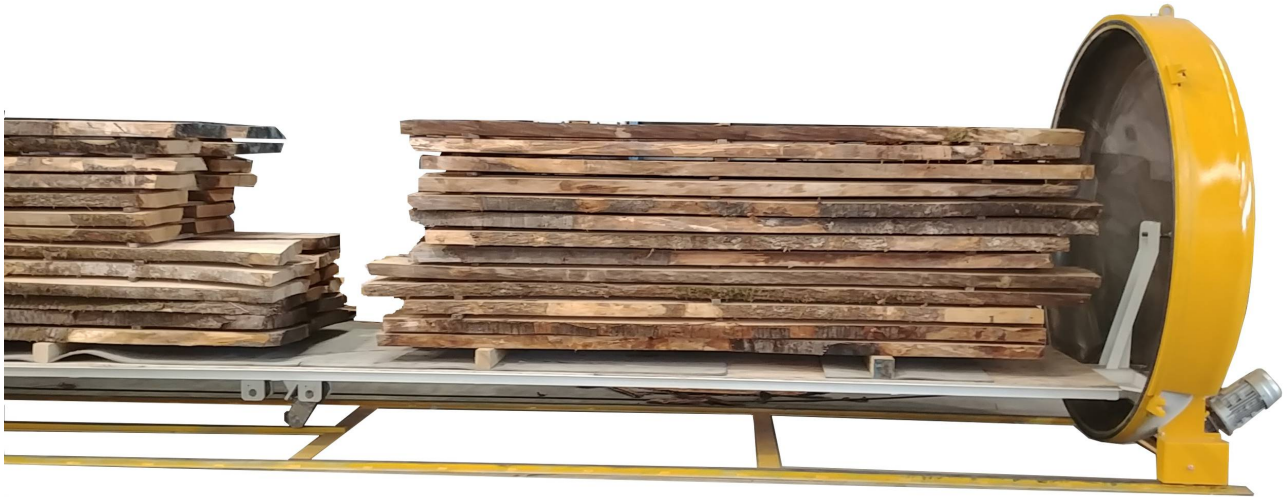
Picture 5.2: charge cart with decked timber ready to be charged on the autoclave
