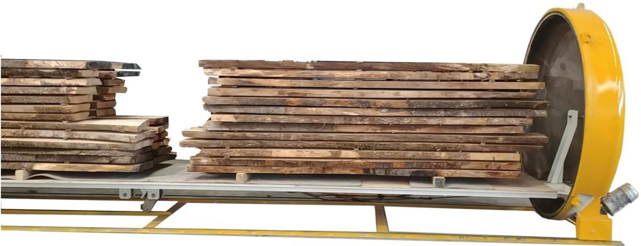
EMV driers can be fitted both of water vacuum pumps and oil ones, the heating system can work with hot water using special radiators or with electricity using heating resistors. Making together one or more oil vacuum pumps and electrical heating system, you can obtain a really versatile machine that needs only EM force lacing and wood water discharge and can be moved easily in case of necessity.
